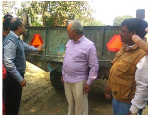
Slow moving vehicle emblem at the rear of tractor and trailer
