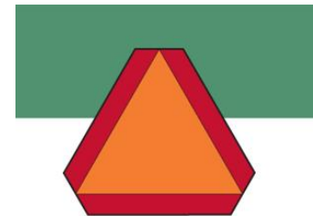
Slow moving vehicle emblem at the rear of tractor and trailer
