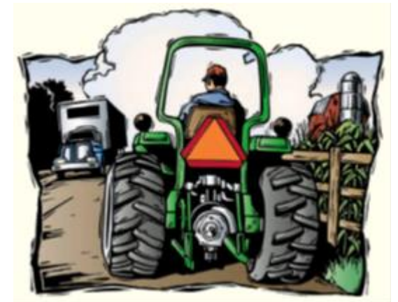
Slow moving vehicle emblem at the rear of tractor and trailer
